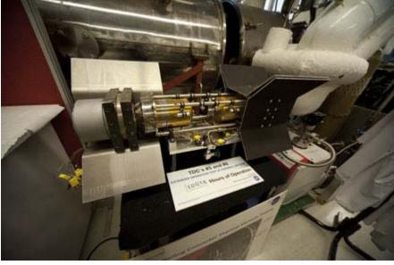
An early ASRG prototype. Its 10,016 hours of use has contributed to decades of combined data on the performance of NASA's revolutionary nuclear battery. (*Dave Mosher/WIRED*) Any hiccups in funding for plutonium-238 production could put planetary science into a tailspin and delay, strip down, or smother nuclear-powered missions. The outlook among scientists is simultaneously optimistic and rattled.
