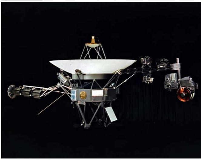
The Voyager probe's three radioisotope thermoelectric generators (RTGs) can be seen mounted end-to-end on the left-extending boom. (*NASA*)
