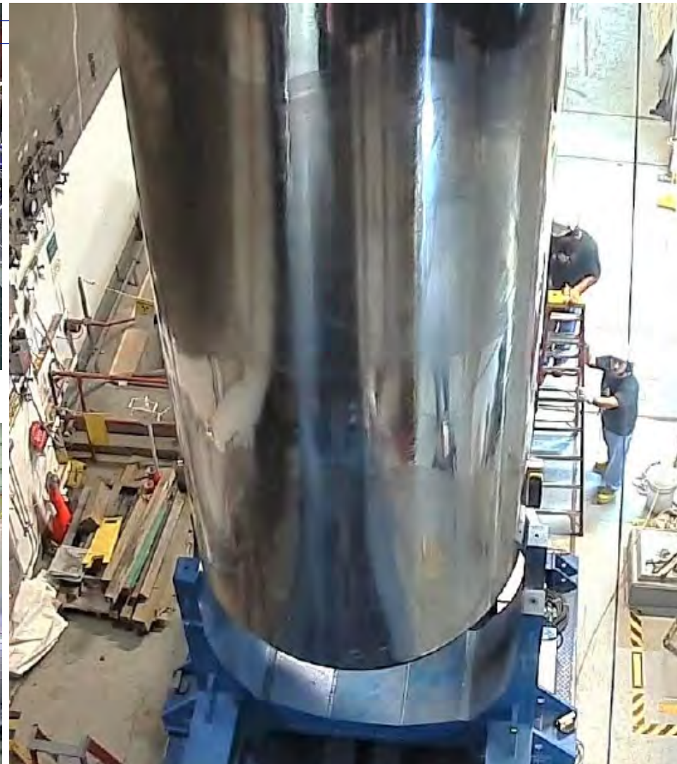
(3) Ready to “down-end” onto Transport Trailer
