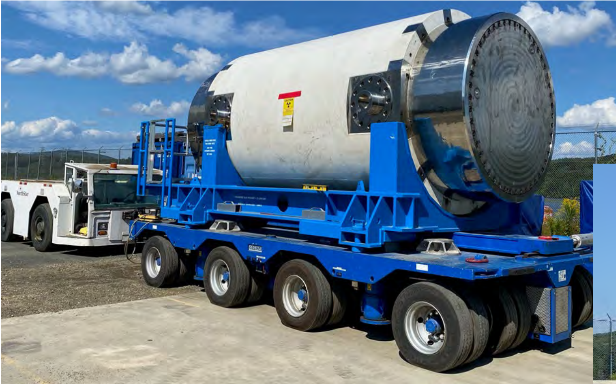
(4) Moving loaded Transfer Trailer with the “Tugger”
