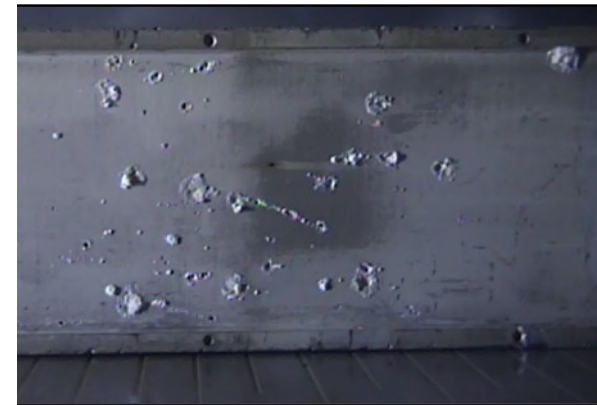
Pitting corrosion on fuel plate
