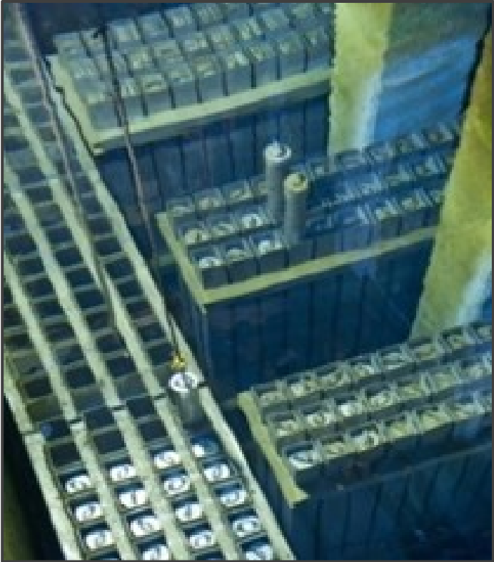
Spent Nuclear Fuel from RR Reactors in Vertical Tube Storage in L Basin
